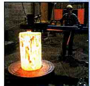
Tool loads hot billets from a hot furnace to a forging press.
