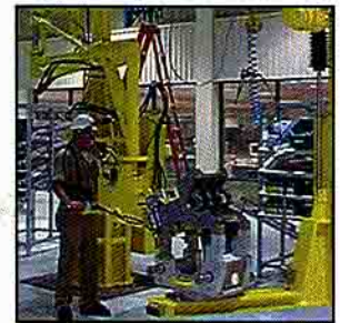
This Taurus loads 400-pound engine blocks onto the final assembly line.
