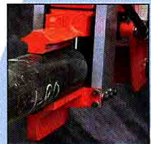
Gripper tool grasps the end of a shaft used in a forging application.
