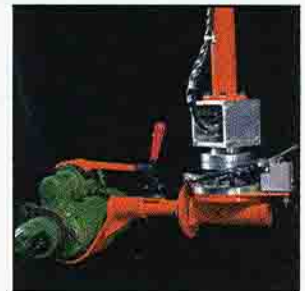
Manually-operated tool picks up 125-pound starters and transfers to the engine during final assembly of a tractor engine.
