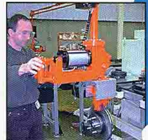
Tool manipulates disk brake hubs through the various manufacturing and machining operations.
