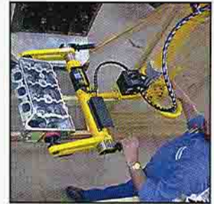
Tool positions engine heads for placement into a 5-axis machining center.
